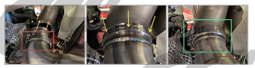
Place the supplied V-band clamp over the end of the downpipe. Match the orientation shown for easy access when tightening
