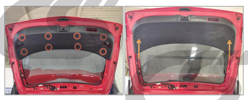
Reinstall the main trim panel by aligning the mounting clips and pressing in the areas circled in the picture.
