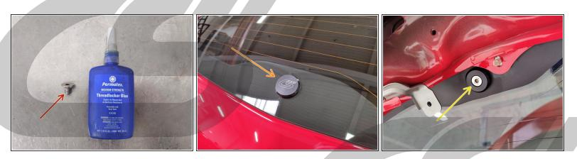
Take the provided M8x12mm Stainless Steel Hex Drive Flat Head Screw and apply Blue Threadlocker.
