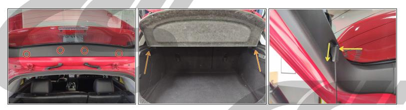
Reinstall the center trim piece by lining up the locking clips and pressing on the locations circled to secure them.
