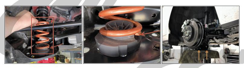
Place the supplied coilover spring onto the OEM perch as shown. Ensure the end of the spring sits against the stop of the OEM perch as shown.
