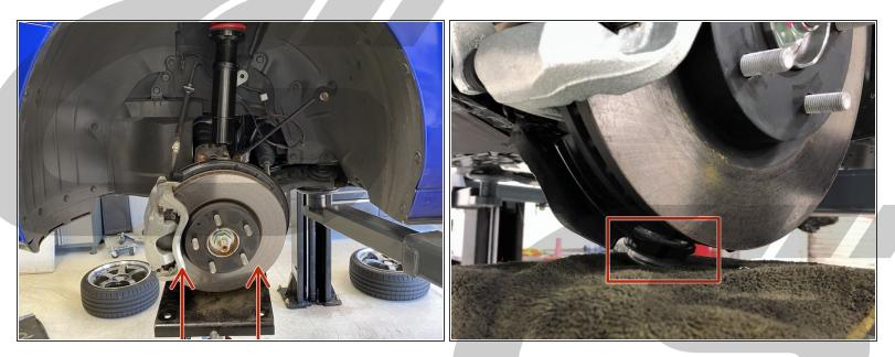
Using a hydraulic jack, lift the knuckle upwards from the lower control arm as shown.
