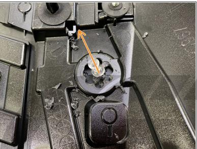
Using your prepared drill bit, drill around the thumb tack until the middle can be removed.
