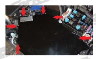
Step 13: Reinstall lid on fuse block (Shown below). Step 14: Reinstall negative battery cable and tighten 10mm nuts on terminal clamps. Step 15: Test drive vehicle. If there is any idling or running issues, recheck the tightness of the hose clamps and that the MAF sensor is fully seated in the MAF housing. ENJOY!!! Thank you for your purchase. If you have any questions please call Cork Sport at 360 260 CORK
