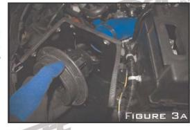
4: INSTALL MAF HOUSING COMPONENTS
