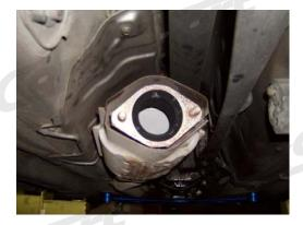
Step 7: Using a hammer, bend the metal on the edge of the tie down hook flat for clearance from exhaust. We recommend protecting the damaged metal with spray paint.
