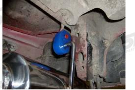
Step 9: Install two (2) supplied washers and two (2) supplied M10 x 1.50 (or M10 x 1.25) thread pitch nuts onto exhaust flange studs and tighten with 17mm wrench or socket.
